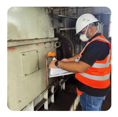
Nanoprecise's MachineDoctor is engineered to go beyond surface-level monitoring. It delivers continuous, high-fidelity data across six critical parameters, enabling earlier detection, deeper insights, and smarter decisions, all in one compact, wireless sensor. Boasting a battery life of up to 8 years and support for WiFi and cellular communication. It is built for flexibility in any environment, no matter how remote or rugged.
