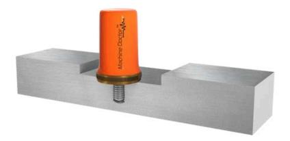
If a pre-threaded hole is not available, the next best option to mount the sensor on the equipment is to apply epoxy at the bottom of the magnet and place it on the equipment. The combination of magnet + epoxy ensures solid bond between the sensors and the equipment.
