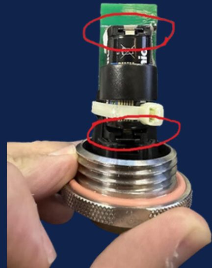
Visual representation of terminals contacting the battery
