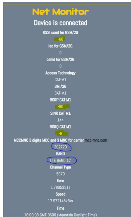
Figure 7: An image detailing connectivity information obtained from the network test sensor via the Nanoprecise provided link.
