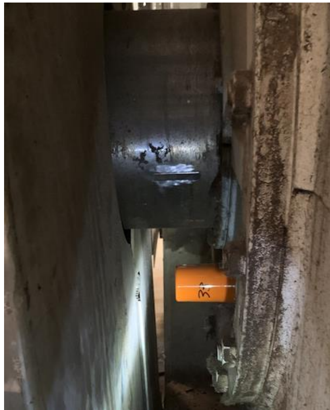
Figure 7 RPM magnet installed with Sensor
